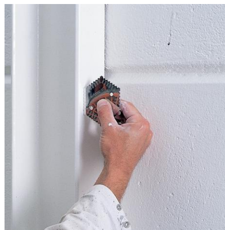
WFT measurements to be recorded regularly.
