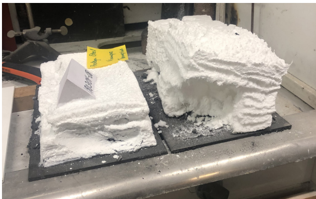
Photograph 1: Intumescent char expansion unrestricted during testing.
