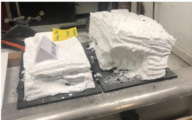
Photograph 1: Intumescent char expansion unrestricted during testing.
